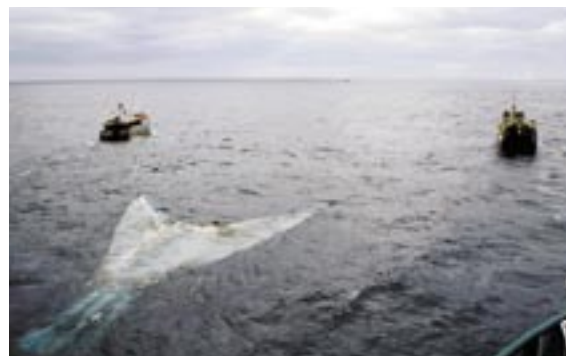
Response means at sea: trawling a slick
