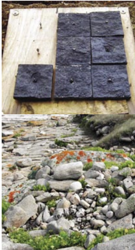
Oiled slabs of granite for a study of oil persistence on rocky substrates (↑) Residual fuel oil from the Erika on a bed of vegetated stones (↓)
