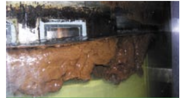
Weathering of oil in Cedre's polludrome* (flume test): formation of a "chocolate mousse"
