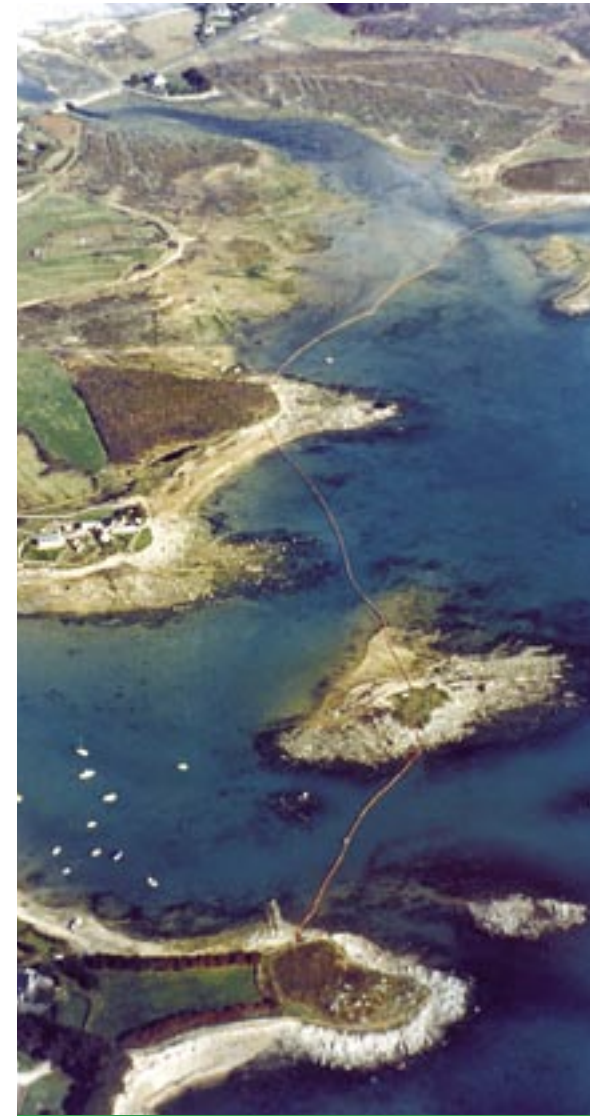
Protecting the port of Ploumanac'h (Brittany, France) during the Tanio pollution using booms
