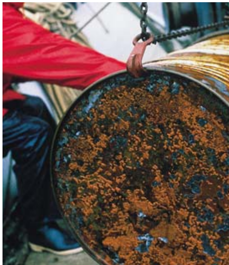
Steel drum after 6 months immersion in sea water (photo Cedre).
