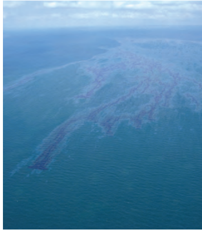
◀ Figure 5: Very large broken slicks of heavy fuel oil – note the absence of sheen. Viewed from 1,000 feet (~300m)
