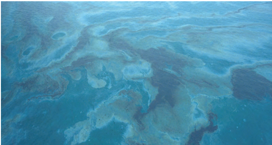
◀ Figure 7: Scattered patches of heavy fuel oil spreading to brown and silver sheen in warm ambient conditions (air temp ~30°C, water temp ~25°C). Viewed from 1,000 feet (~300m)
